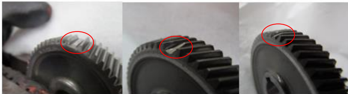
Figure 1: Three level of fault severity. Left to right: removal of 25% of the tooth's width, removal of 50%, and a missing tooth.
