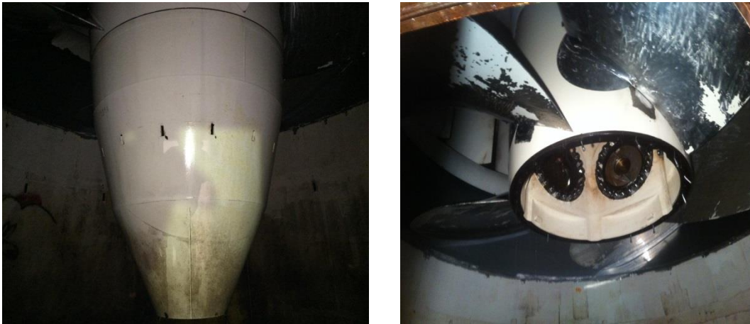
Figure 6: View of the propeller runner cone, before (left) and after (right) the loss
