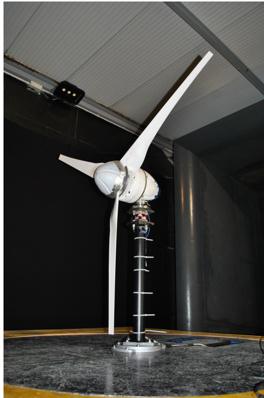
Figure 1: The small HAWT in the wind tunnel open test section.
