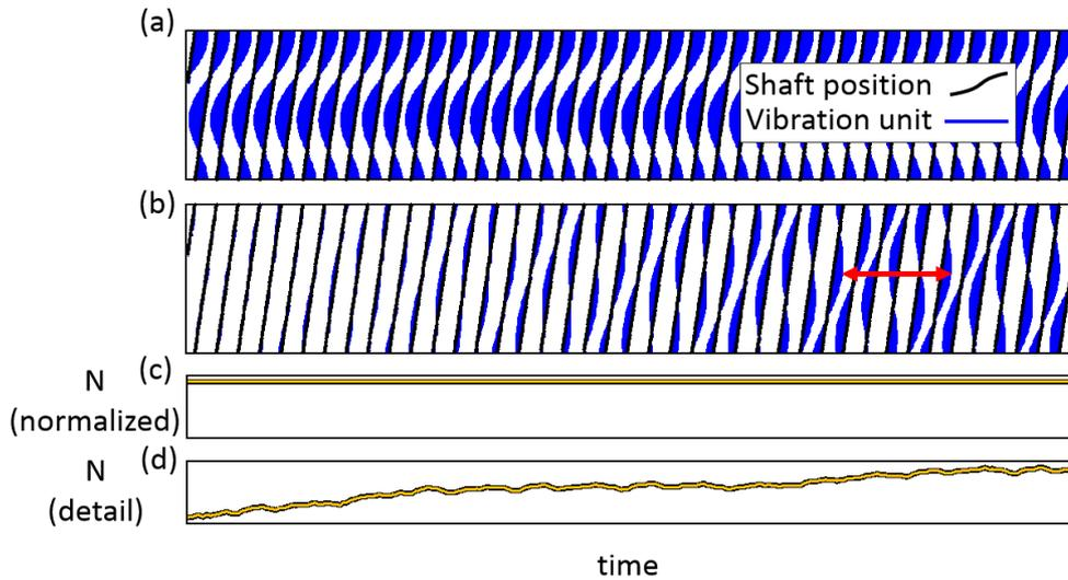
Figure 3: Application to a constant rigid unbalance and the progressive increase of an oil unbalance. Representation in the time/phase domain of the vibration amplitude tracked on the first order 1 N of the rotating speed (a) and of the vibration amplitude tracked around 0.8 N (b). Time history of the normalized rotating speed (c) and of the detail of the rotating speed (d). The red arrow shows that it takes 5 rotations of the shaft for the oil unbalance to be repetitive.
