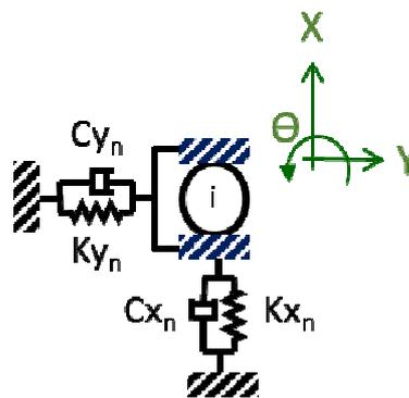
Figure 10: Lumped mass model Schema.
