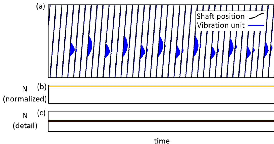
Figure 14: Simulation of the response to repetitive shocks. Representation in the time/phase domain of the vibration amplitude of an accelerometer mounted on a case of the engine (a). Time history of the normalized rotating speed (b) and of the detail of the rotating speed (c).
