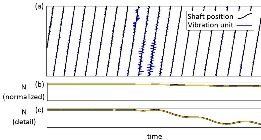
Figure 7: Application to a compressor stall. Representation in the time/phase domain of the vibration amplitude of an accelerometer mounted on a stator close to the shaft (a). Time history of the normalized rotating speed (b) and of the detail of the rotating speed (c).
