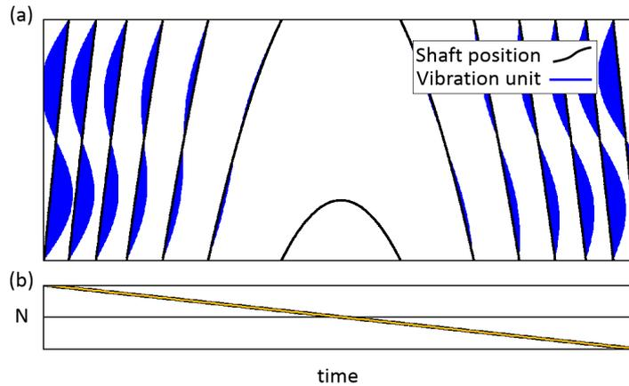
Figure 2: Representation in the time/phase domain (a) and time history of the shaft rotating speed (b).
