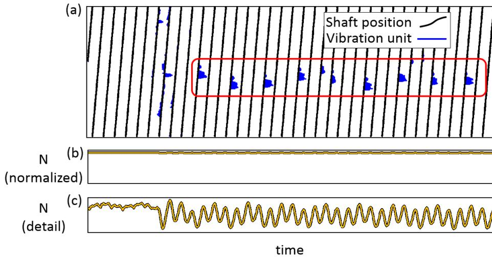
Figure 9: Repetitive shocks on a static case when a rotor interacts with a stator. Representation in the time/phase domain of the vibration amplitude of an accelerometer mounted on a case of the engine (a). Time history of the normalized rotating speed (b) and of the detail of the rotating speed (c).
