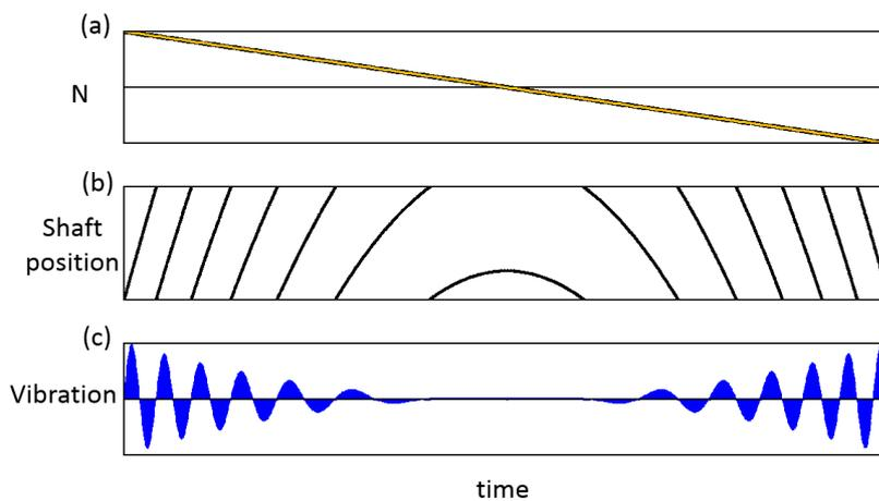
Figure 1: Standard time history representation with a simple simulation. Time history of the rotating speed  $N$  of a shaft (a), time history of the shaft angular position (b), and time history of a simulated vibration signal (c).
