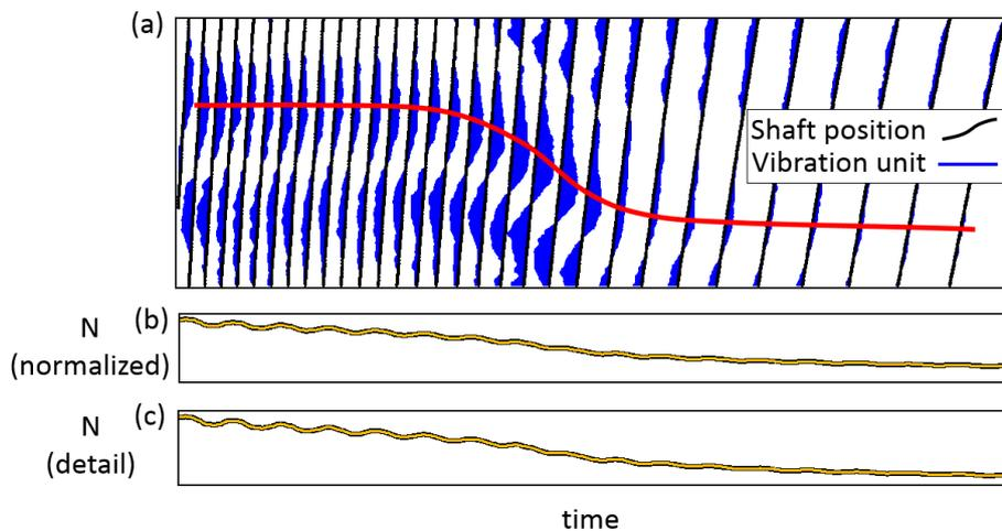
Figure 8: Application to the crossing of the rotating speed and a mode of the shaft. Representation in the time/phase domain of the vibration amplitude of a strain gauge mounted on a stator close to the shaft (a). Time history of the normalized rotating speed (b) and of the detail of the rotating speed (c). The red curve follows the maximal positive amplitude at each cycle.
