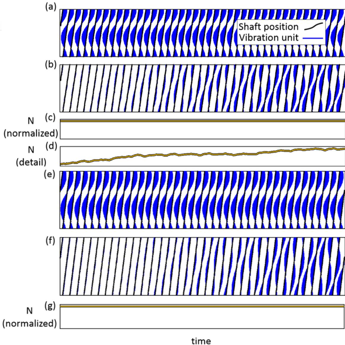
Figure 11: Application to a constant rigid unbalance and the progressive increase of an oil unbalance. Representation in the time/phase domain of the vibration amplitude tracked on the first order 1 N of the rotating speed (measurement (a), simulation (e)) and of the vibration amplitude tracked around 0.8 N (measurement (b), simulation (f)). Time history of the normalized rotating speed (measurement (c), simulation (g)) and of the detail of the rotating speed for the measurement (d).
