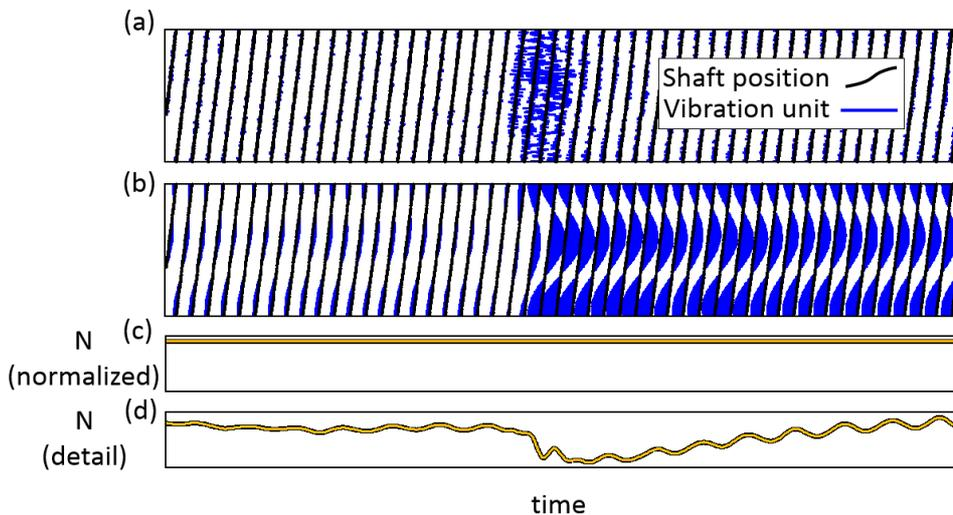
Figure 4: Application to ice shedding, fleeting event and sustained unbalance. Representation in the time/phase domain of the vibration amplitude (a) and of the vibration amplitude tracked around 1 N (b). Time history of the normalized rotating speed (c) and of the detail of the rotating speed (d). The unbalance increases in amplitude during the shedding while preserving its phase location.
