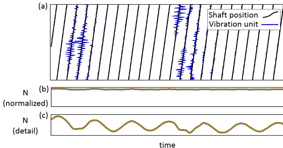
Figure 6: Application to the ingestions of several birds. Representation in the time/phase domain of the vibration amplitude of an accelerometer mounted on a stator close to the shaft (a). Time history of the normalized rotating speed (b) and of the detail of the rotating speed (c).
