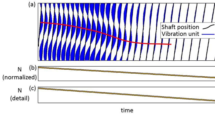
Figure 12: Simulation of the response to a crossing of the rotating speed and a mode of the shaft. Representation in the time/phase domain of the vibration amplitude of a strain gauge mounted on a stator close to the shaft (a). Time history of the normalized rotating speed (b) and of the detail of the rotating speed (c). The red curve follows the maximal positive amplitude at each cycle.
