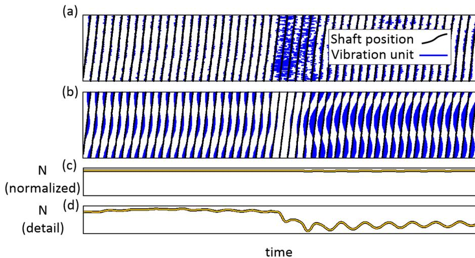
Figure 5: Application to ice shedding, fleeting event and change in unbalance amplitude and position. Representation in the time/phase domain of the vibration amplitude (a) and of the vibration amplitude tracked around 1 N (b). Time history of the normalized rotating speed (c) and of the detail of the rotating speed (d). The unbalance decreases and increases in amplitude during the shedding while its phase location is almost at the opposite direction.
