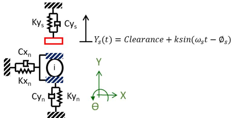
Figure 13: Rotor-stator contact model schema.
