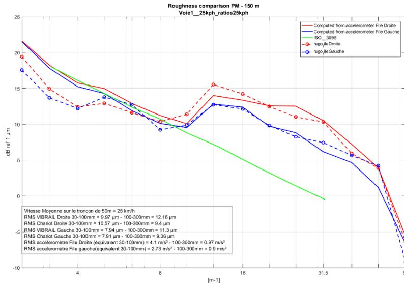
Figure 4 : 1 Third octave spectra (in 1/m) measured (with trolley in dashed lines) and computed (with inverse method in solid lines). In green, the ISO 3095 standard
