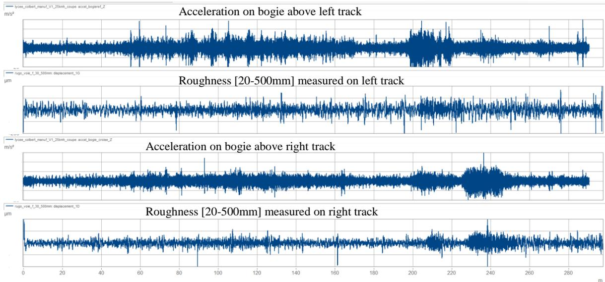
Figure 3: Accelerations measured on a bogie and roughness on the same portion of track at 25 km/h
