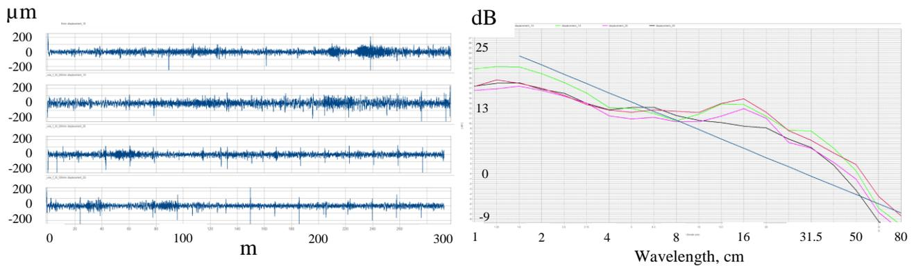
Figure 2: Left side: roughness in  $\mu\text{m}$  measured on 4 track lines.
