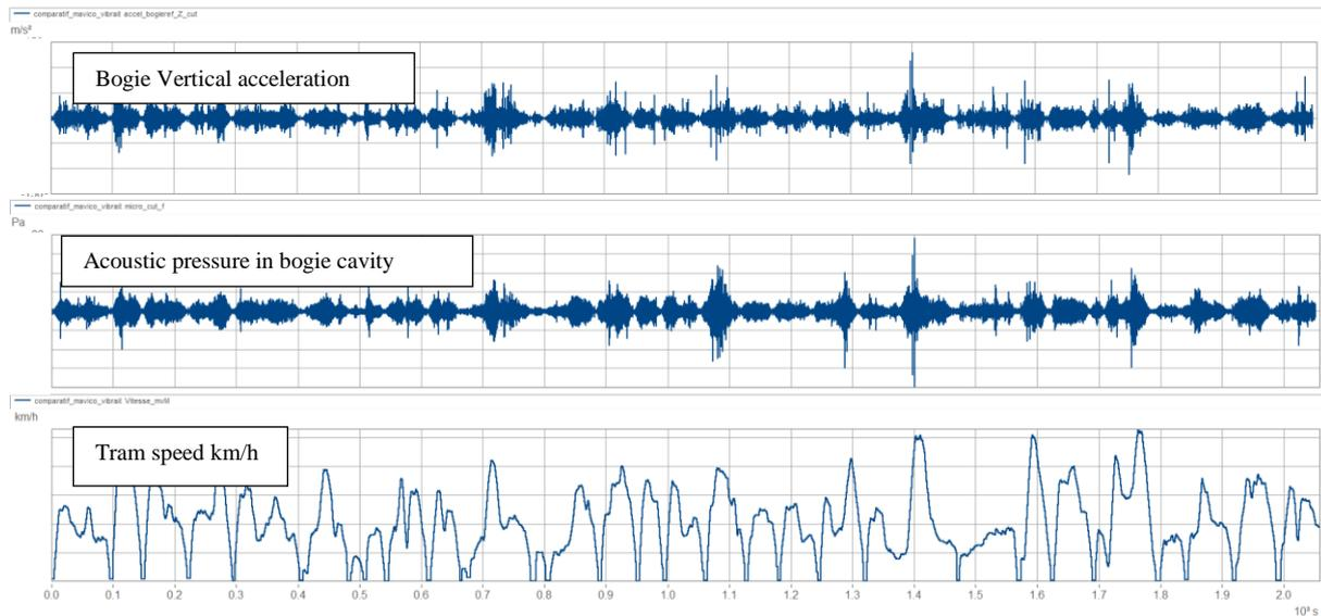
Figure 8: raw data measured by the device on the Lyon tramway network T1 Line
