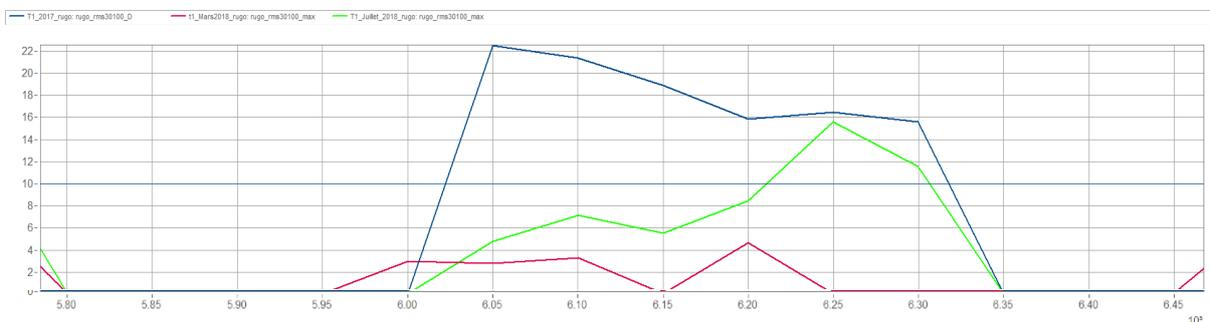
Figure 13: rail roughness - RMS level in the [30-150]mm wavelength. Status July 2017, Status March 2018, Status July 2018
