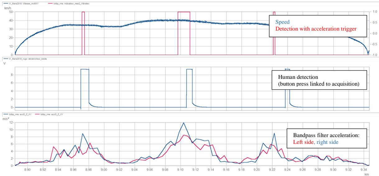
Figure 10: correlation between bandpass filtered acceleration and human detection on an interstation
