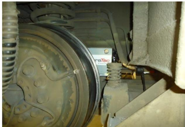
Figure 7: localisation of VibRail Concept n°1 on a tramway bogie
