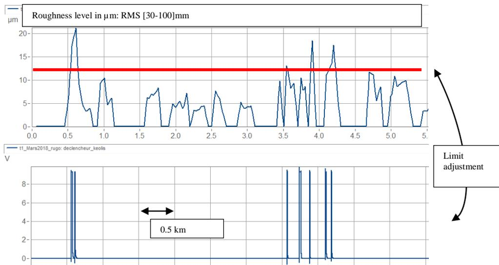
Figure 12: Top: Rail roughness - RMS level in the [30-150]mm wavelength. Bottom: Correlation with subjective detection
