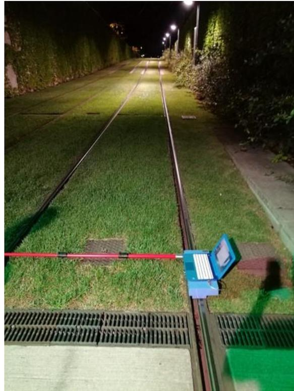
Figure 1: rail corrugation analysis trolley
