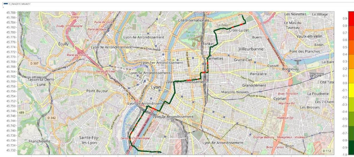
Figure 11: Example of a GPS map of the roughness level (Lyon tramway network T1 Line).
