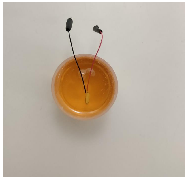
Fig. 3. Specimen of epoxy resin curing monitoring
