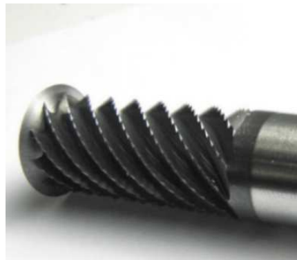
Figure 2: Milling cutter used for Nomex ® honeycomb core “CZ10”.
