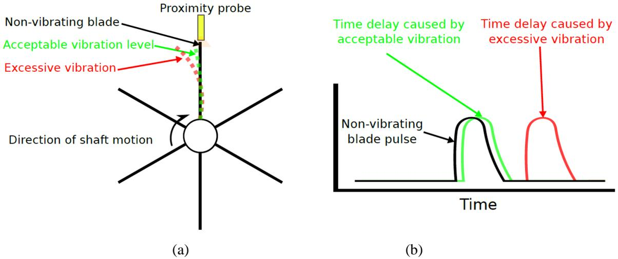
Figure 2: Blade tip timing (a) Rotor blade during operation (b) Proximity probe output
