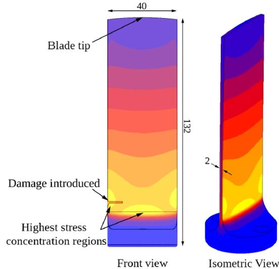
Figure 5: Damage introduced on blade 2, relative to the areas of highest stress concentration for mode 1, as determined from a FEA
