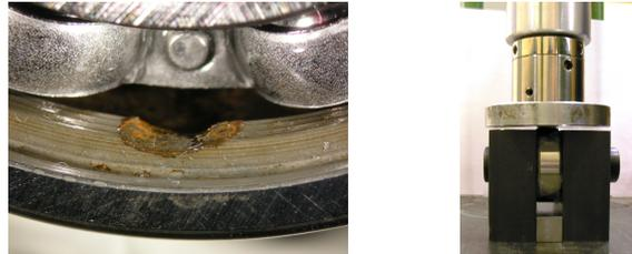
Figure 3: Micrograph of the chemically etched outer race defect (left). Photo of the hydraulic press employed to impart bearing brinelling damage (right).
