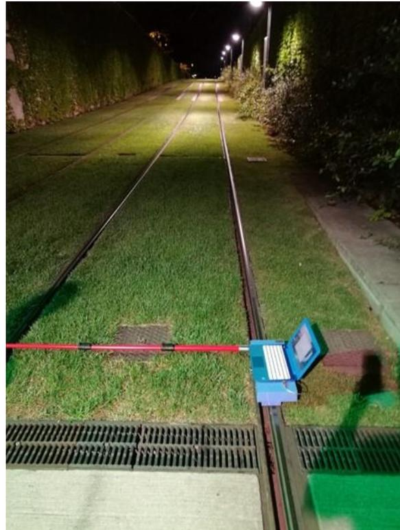
Figure 1: rail corrugation analysis trolley
