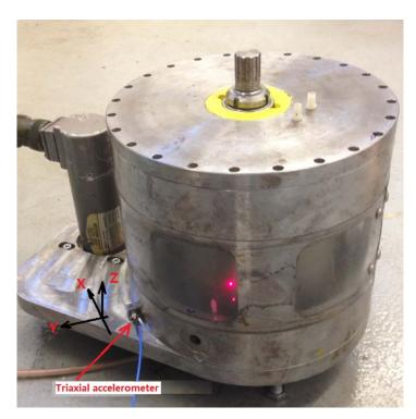
Figure 7. Electrorheological torsional absorber
