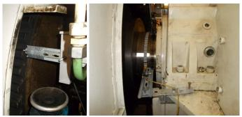
Speed measurements on the engine and on the generator
