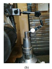
Figure 8: (a) Experimental setup of the grinding machine, (b) Emulation of an eccentric workpiece.
