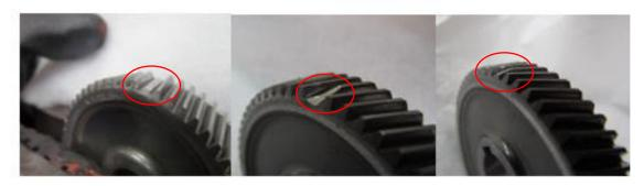
Figure 1: Three level of fault severity. Left to right: removal of 25% of the tooth's width, removal of 50%, and a missing tooth.
