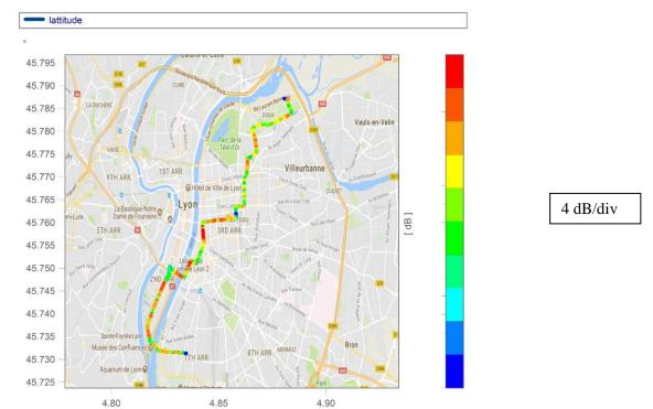
Figure 9: Lyon tramway network T1 Line. GSP track, with a color scale corresponding to RMS acoustic pressure under the bogie in dB
