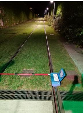
Figure 1: rail corrugation analysis trolley
