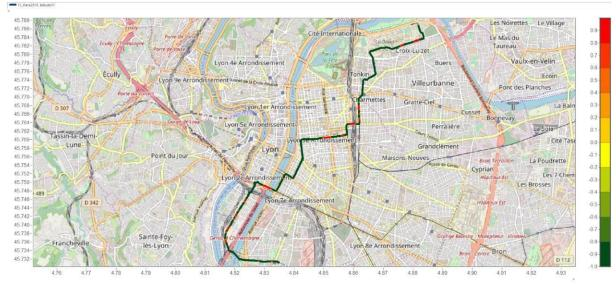
Figure 11: Example of a GPS map of the roughness level (Lyon tramway network T1 Line).
