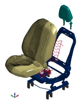
Figure 3: Exploded view of the complete seat finite element model.
