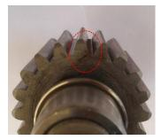
Figure 6 : Planet gear with tooth root crack
