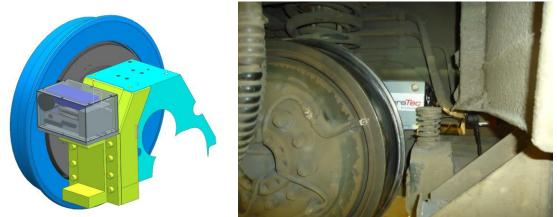
Figure 7: localisation of VibRail Concept n°1 on a tramway bogie
