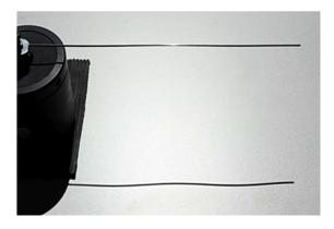
A cantilever beam is excited by a shaker with a swept sine. Contestants shall perform the modal analysis of the beam from the video file.
