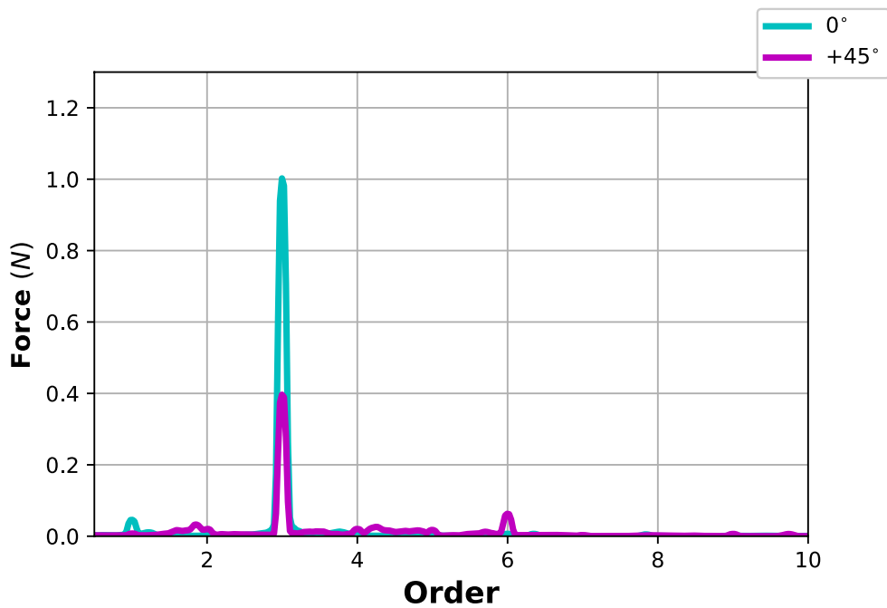
Figure 2 Experimental normalized order spectrum of the forces (fore-aft component normalized on the amplitude of the 3P component with zero yaw).
